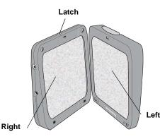
1. While holding the latch on the top of the right speaker, pull the speaker halves apart to separate them.
